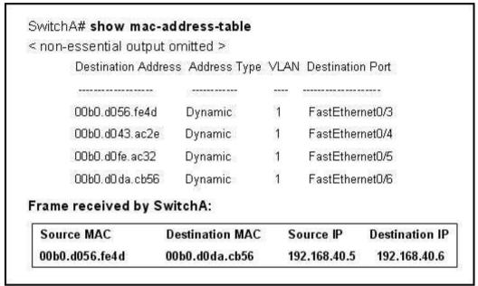
SwitchA receives the frame with the addressing shown. According to the command output also shown in the exhibit, how will SwitchA handle this frame?
