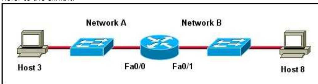
Host 3 on Network A is sending data to Host 8 on Network B. Which address is the default gateway of Host 3?
