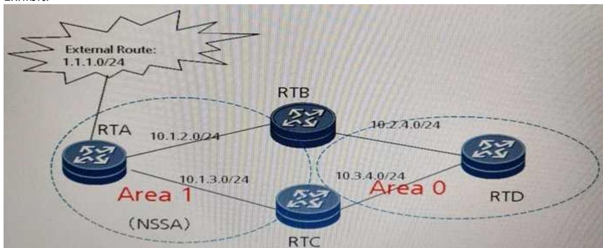
As shown in the figure, external route 1.1.1.0/24 is imported to RTA that is located in the NSSA area. RTD is a backbone area router. RTB and RTC are both area border routers (ABRs). OSPF configuration is as follows.
