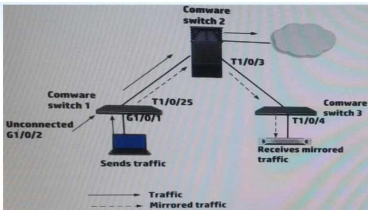
A network administrator up a remote mirroring on the HP Comwaer switches in the exhibit. The administrator must define several port while entering mirroring-group commands on these switches.
