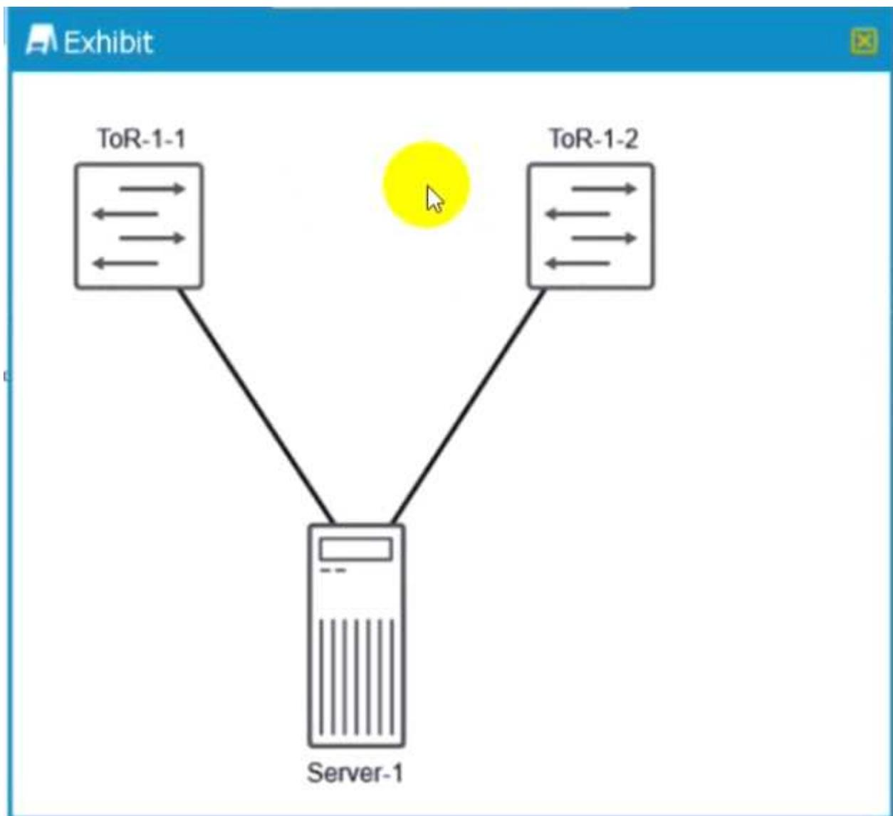
You are designing a data center where all your servers in each rack will be connected to two top-of-rack (ToR) switches using Layer 2 as shown in the exhibit. You must implement a high availability solution that maintains link layer connectivity to each server when one of the ToR switches fails. In this scenario, which solution will accomplish this task?
