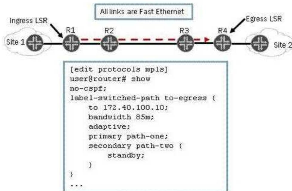
As shown in the exhibit, you have an adaptive LSP that requires 85 Mbps. The LSP is configured with a primary path and a secondary path in standby mode. All connections in the MPLS network are Fast Ethernet. Which statement is correct?
