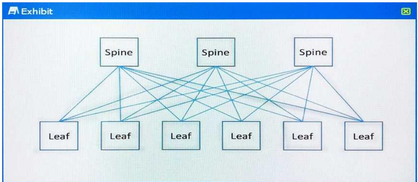
A customer has a 3-stage Clos architecture with three spine devices as shown in the exhibit. If a single spine device fails, what percentage of the remaining bandwidth will be available from leaf node to leaf node?
